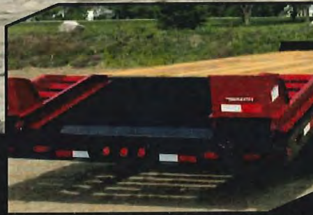
Self-cleaning angle iron beaver tail also provides positive traction when loading equipment.
