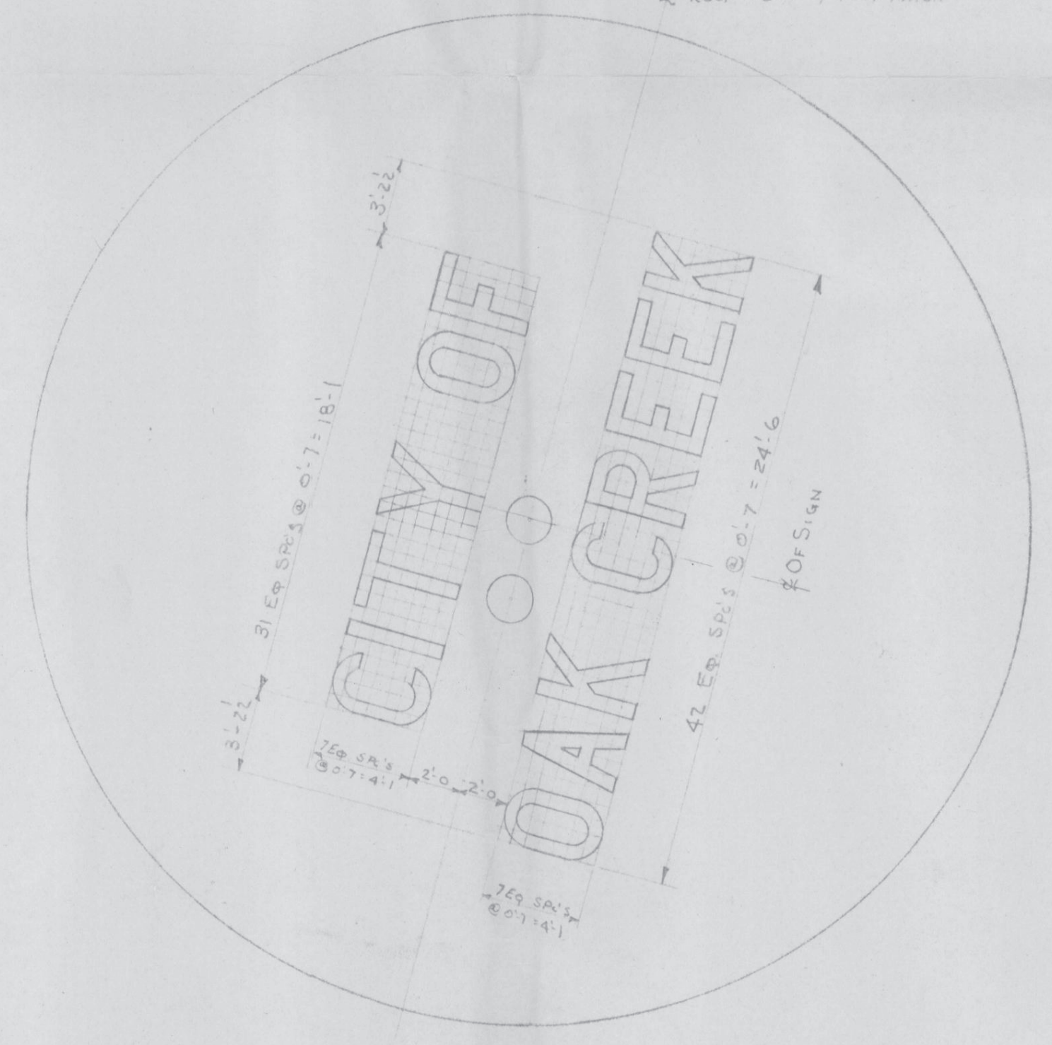
SIGN AT TOP OF TANK
